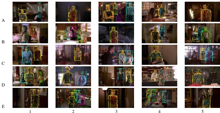
Figure 3: Typical results on the Buffy data set. Positive detections are overlaid with the learnt HOG template of the corresponding model, deformed by the deformation field. Large majority of the persons are correctly detected. Typical mistakes include missed detections of hard instances (A3, A4, C3, E4), false positive detections (A5, B2), detection with insufficient overlap with the ground truth (B3) or detection by a wrong model with a wrong truncation (A3).
