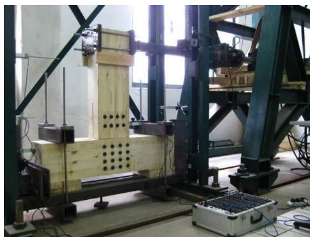
Fig. 10 Test setup for the joint connection
