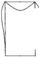
(a) Local Buckling
