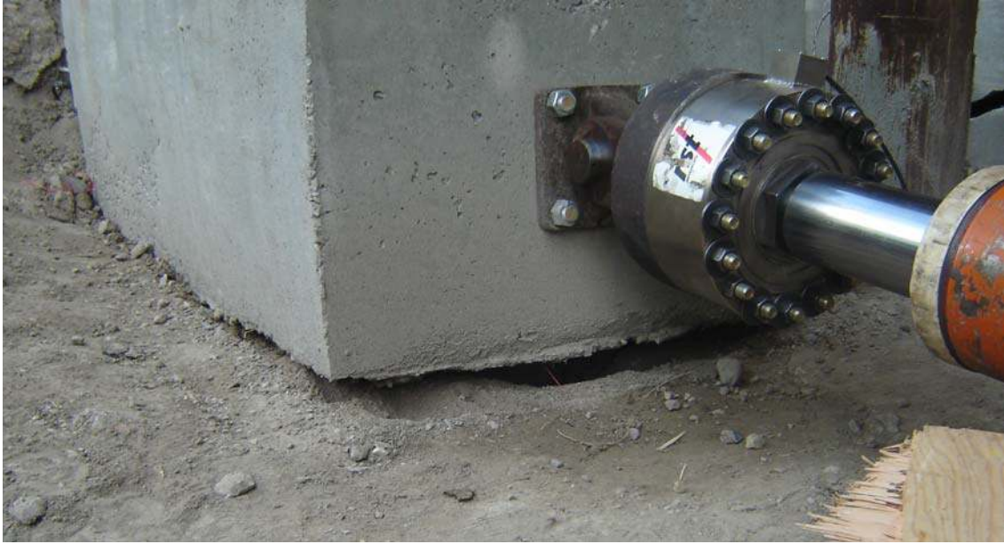
Figure 5-18 Test Cap 4 at failure.
