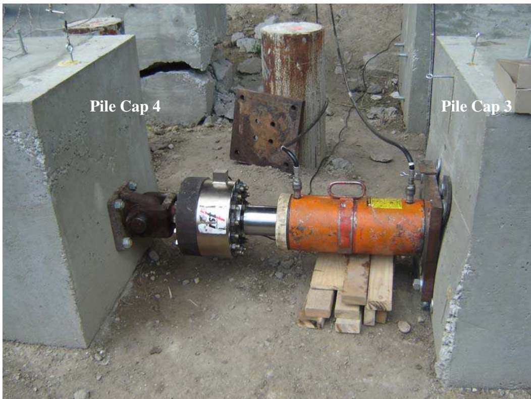
Figure 3-20 Photograph of test layout for test on Pile Cap 4.
