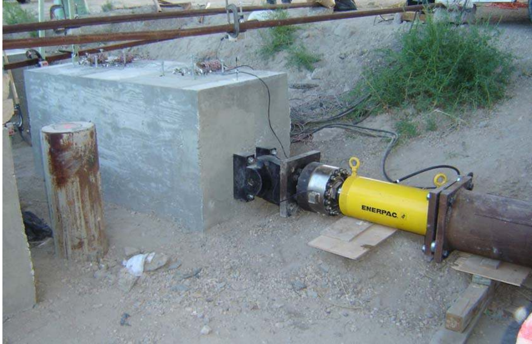
Figure 3-16 Photograph of test set-up for Pile Cap 2.
