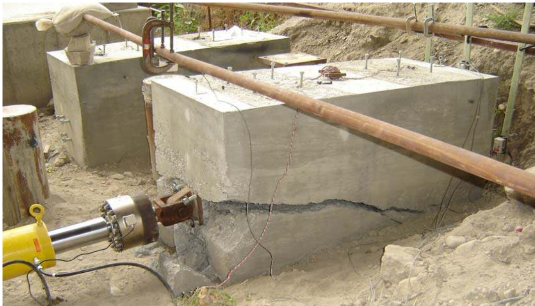
Figure 5-14 Test Cap 3 at failure.
