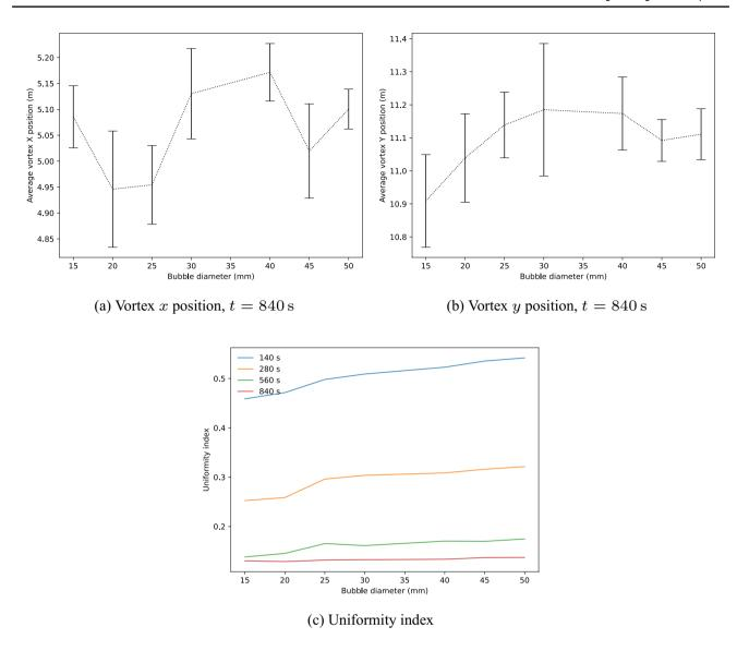
**Fig. 12** Dependence on bubble size. "Sparse" results,  $n_x = 80$ , 2.5% TS sludge
