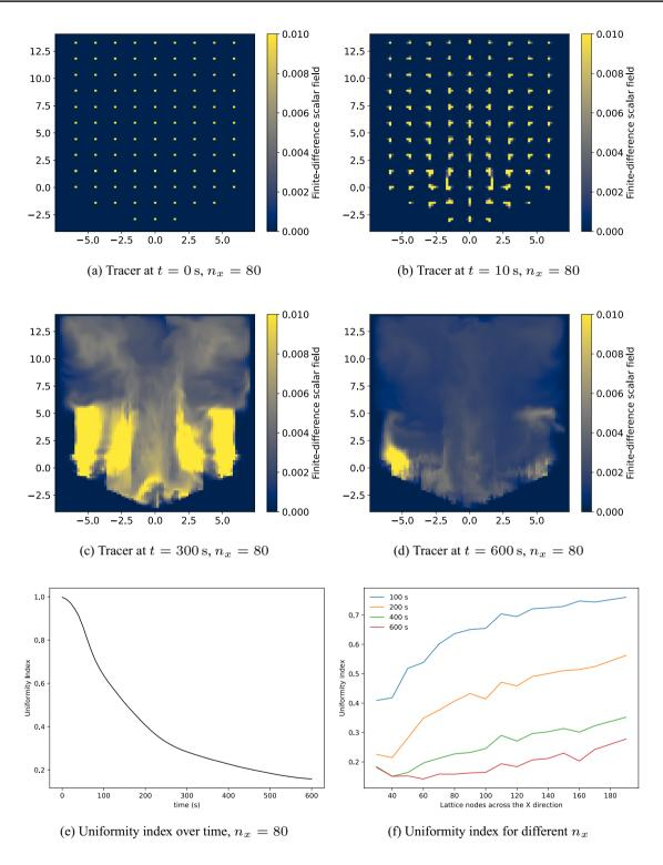
Fig. 7 "Sparse" results, 2.5% TS sludge, 50 mm bubble size
