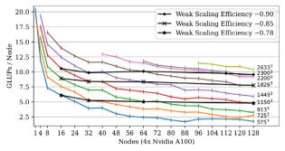
(a) Scalability of OpenLB 1.5 on HoreKa (multi-GPU execution MPI & CUDA) up to the max. number of nodes allocatable [58]. Throughput in giga  $(10^9)$  lattice (cells) updates per second (GLUPs) on the y-axis, for resolutions (N per coordinate axis) labeled on the right.
