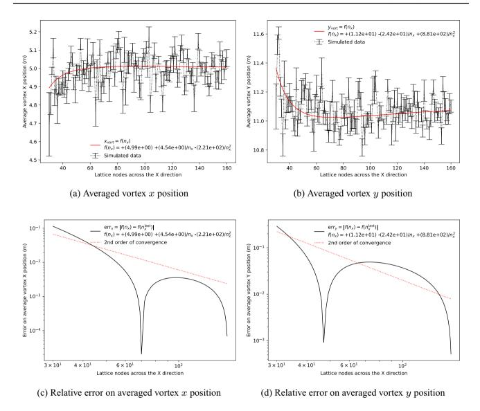
Fig. 6 Averaged vortex position and relative error, 2.5% TS sludge, 50 mm bubble size. Average performed for  $t \ge 200$  s
