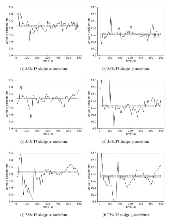
Fig. 4 Vortex coordinates over time,  $n_x = 80$ , 50 mm bubble size. Solid lines: instantaneous values. Dashed lines: averages, computed from 200 s onwards. Dotted lines: statistical standard errors computed from adapted standard deviations, computed from 200 s onwards
