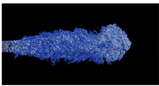
(b) Q-Criterion iso-contours of GPU-based 3D turbulent nozzle flow simulation using 2.5 billion cells [58]. Colours indicate velocity magnitude from low (blue) to high (orange).
