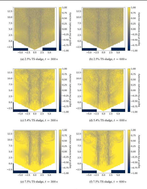
Fig. 5 Apparent viscosity over characteristic viscosity,  $n_x = 80,50 \,\mathrm{mm}$  bubble size
