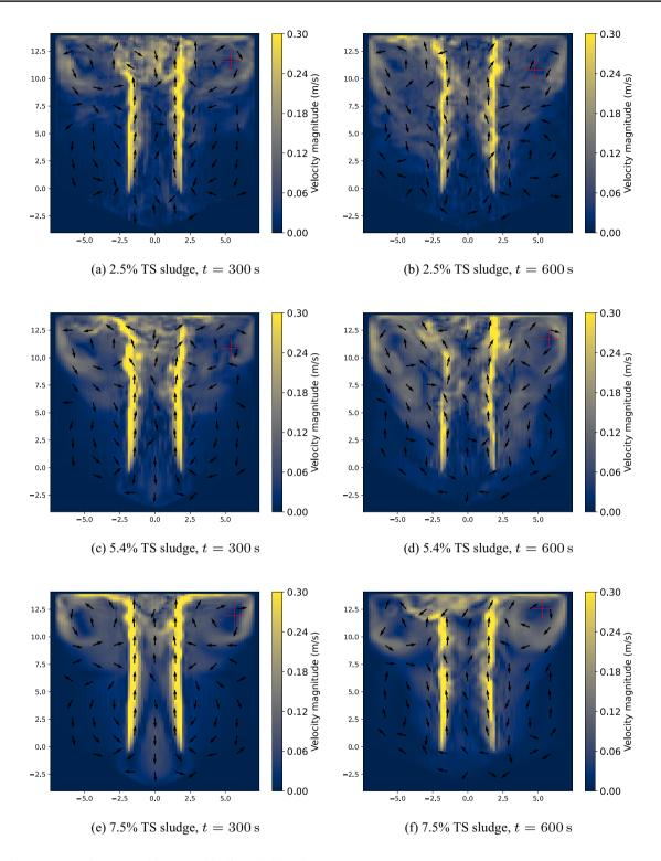
Fig. 3 Flow patterns and vortex position,  $n_x = 80, 50 \,\mathrm{mm}$  bubble size
