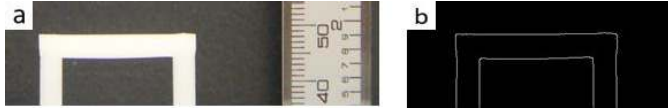
Fig. 13. Image analysis of the horizontal strut. (a) Original image. (b) Sharpened image for edge detection.
