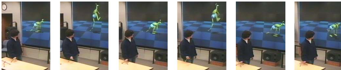
Figure 1: While watching a real-time display of her actions, an animator performs a hopping motion, sketching the trajectory of a kangaroo.
