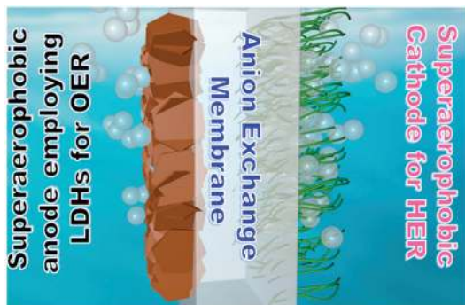
Fig. 24 Schematic illustration of the proposed “ideal” MEA (membrane–electrode assembly) with both the anode and cathode having nanoarray structures and being superaerophobic for efficient water splitting that includes the OER at the anode and the HER (hydrogen evolution reaction) at the cathode.
