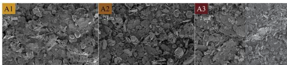
Figure 17. SEM micrographs of the chemical morphology/crystallinity of \text{Al}(\text{OH})_3 series A1 = SA, A2 = ACE and A3 = M taken at 1 keV and 2k magnification. The scale bar is indicated below the label.
