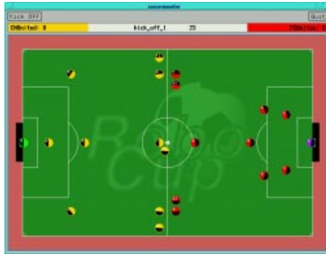
Figure 2.1: The soccer server display. Each player is represented as a two-halved circle. The light side is the side towards which the player is facing. All players are facing the ball, which is in the middle of the field. The black bars on the left and right sides of the field are the goals.
