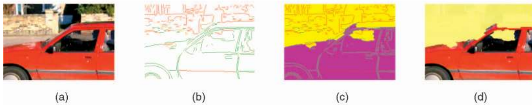
Fig. 9. “Car” segmentation from two frames. (a) Original frame. (b) Edge labels after EM. (c) Most likely region labeling. (d) Final foreground segmentation.
