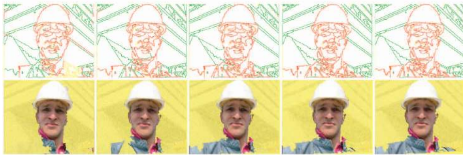
Fig. 11. Evolution of the “Foreman” segmentation, showing the edge probabilities and segmentations of frame 1 as the evidence is accumulated over five successive frames. The edge probabilities become more certain and small errors are removed, resulting in an improved region segmentation.
