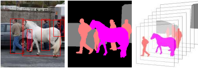
Fig. 1. Multi-class object detections algorithms typically predict bounding box locations and class labels (left) but this only provides coarse information about object localization. We propose to use object detector outputs to guide multi-class segmentation algorithms that provide class labels for every pixel (center). To do so, we introduce layered representations (right) that reason about relative depth orderings of detected objects and can link disconnected object segments separated by an occluder (e.g., the feet and head of the center person occluded by the horse).
