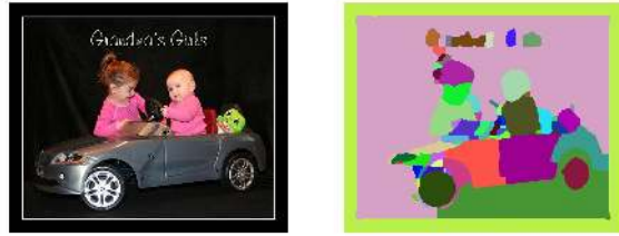
Fig. 4. An example superpixel grouping from [33] tuned to return roughly 200 superpixels. We use this bottom-up information in our probabilistic model by constraining all pixels within a superpixel to share the same label.
