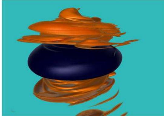
FIGURE 10. Three-dimensional perspective of vortex stretching at day 200 of run A: the blue isosurface corresponds to non-dimensional value of -0.4 and the orange isosurface to a non-dimensional value of +0.3 .
