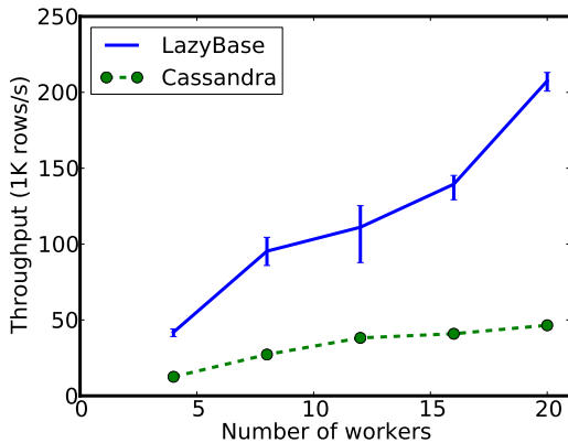
Figure 3. Inserts processed per second. Error bars represent the min and max of three runs, while the line plots the mean.
