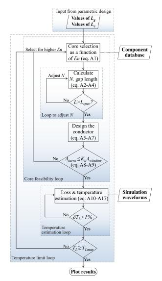
Figure A1. Inductor hardware design flowchart.
