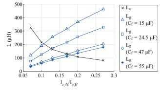
**Figure 3.** Inductance of  $L_c$  and  $L_g$  as a function of  $I_{c,f_s}/I_{c,lf}$ , for different  $C_f$ .
