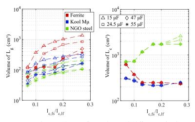
**Figure 4.** Inductor volumes of  $L_c$  and  $L_g$  with different technologies as a function of  $I_{c,f_s}/I_{c,lf}$ , for different  $C_f$ .
