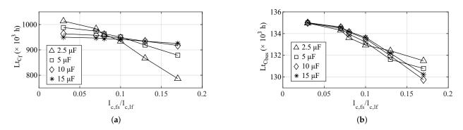
**Figure 11.** Estimated capacitor lifetimes as a function of  $I_{c,f_s}/I_{c,lf}$ . (a)  $Lt_{C_f}$ . (b)  $Lt_{C_{bus}}$ .
