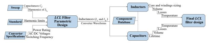
Figure 1. Diagram illustrating the developed methodology.
