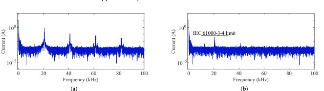
In Figure 13 the harmonic amplitudes of current over the frequency spectrum in  $L_c$  and  $L_g$  are presented. The measured ratio of  $I_{g,f_s}/I_{g,l_f}$  is of 0.41%, close to the stipulated value of approximately 0.4%.
