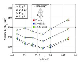
**Figure 5.** Technologies that result in smallest combined volume of  $L_c + L_g$ , as a function of  $I_{c,f_s}/I_{c,lf}$ , for different  $C_f$ .
