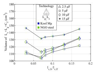
**Figure 10.** Total filter volume:  $L_c + L_g + C_f$ , as a function of  $I_{c,f_s} / I_{c,lf}$ , for the converter from Table 2.
