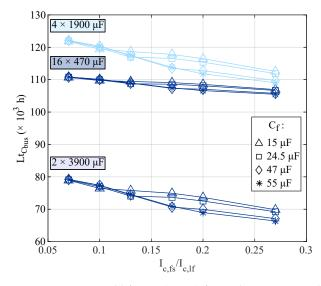
**Figure 8.** Estimated lifetime ( $Lt_{C_{hus}}$ ) for each capacitor in the DC bus, as a function of  $I_{c,f_s}/I_{c,l_f}$ .
