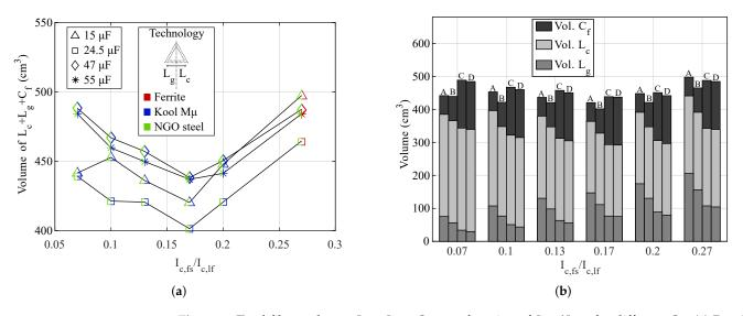
**Figure 6.** Total filter volume:  $L_c + L_g + C_f$ , as a function of  $I_{c,f_s} / I_{c,lf}$ , for different  $C_f$ . (a) Results identifying inductor technology. (b) Individual component volumes, where each bar represents an analyzed value of  $C_f$ , in ascending order: (A) 15  $\mu$ F; (B) 24.5  $\mu$ F; (C) 47  $\mu$ F; (D) 55  $\mu$ F.
