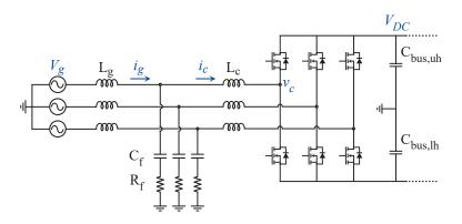
Figure 2. Converter topology: input stage of double-conversion UPS with common neutral point connection.
