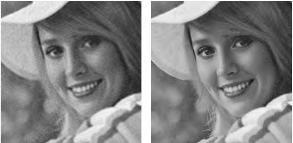
Fig. 22. A fragment of the reconstructed “Elaine” image after the applications of: Left: JP2k . Right: RLCTA/8/8+SPIHT . The compression ratio is 1/4 bit per pixel.
