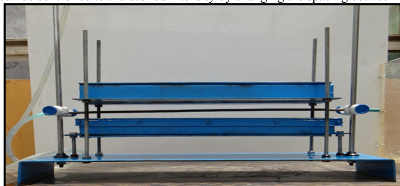
Figure 2. The variable intensity magnetization device.
