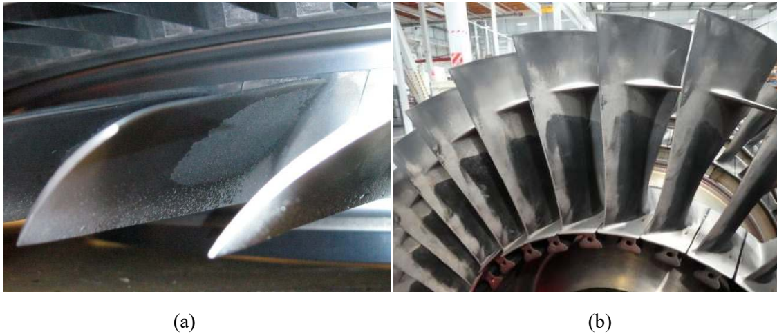
Figure 22 Deposits on Low-pressure compressor (LPC) stage 2.5 blades and on High-pressure compressor (HPC) stage 3 blade [98]
