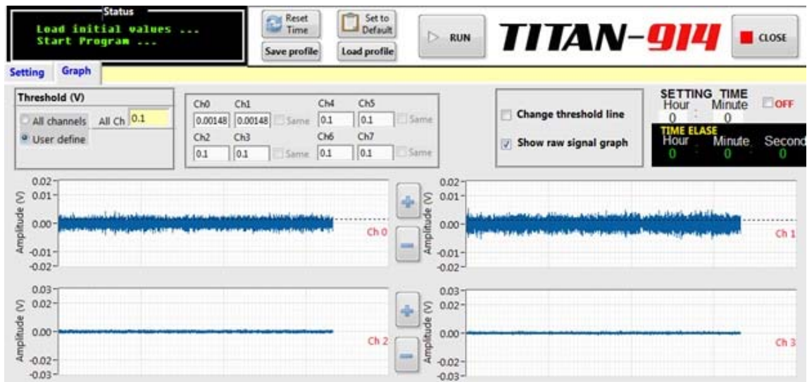
Fig. 6. Time domain waveform of the leaking location at 3.0 m
