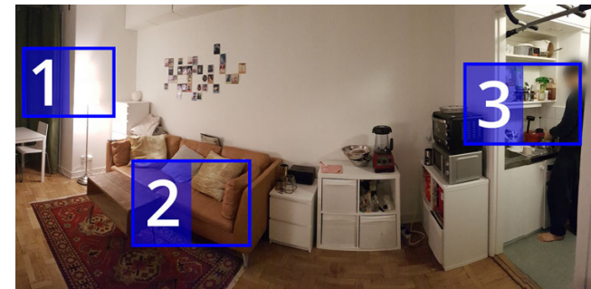
Figure 1: Diagram of sensor locations in our studio apartment. A photocell (remains) is within the floor lamp (1), a soft potentiometer (removed) was tried in various couch locations (2), and a temperature sensor (removed) was above the stove (3).
