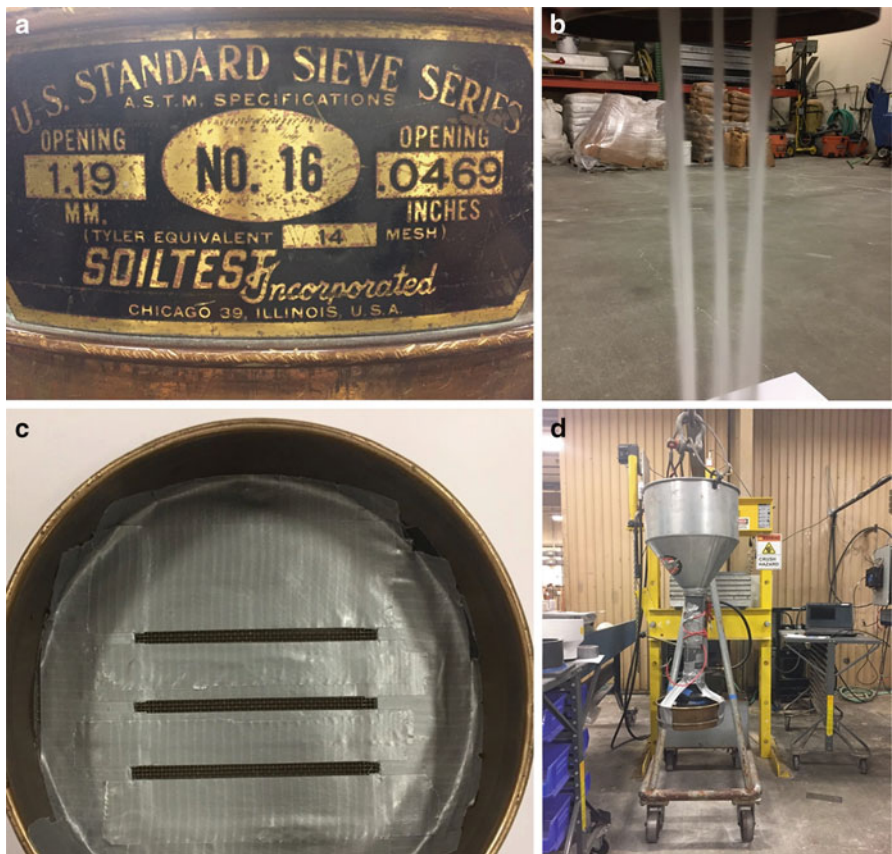
Fig. 1.1 (a) Standard sieve used for calibration tests in this specification. (b) Side view of sand falling for 7.1 mm slots spaced at 17 mm. (c) Duct tape used to mask off slots for pluviation; the 7.1 mm slots correspond to three mesh widths of the standard sieve. (d) Ad hoc arrangement of sieve attached to hopper used to feed sand to the sieve during pluviation
