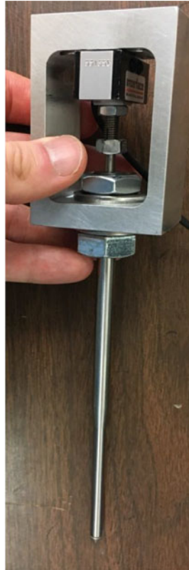
Fig. 1.11 Images of a new design for LEAP-2017 CPT device and rod lengths of the devices used at different facilities
