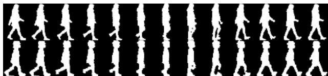
FIGURE 3. Period-normalized phase-synchronized silhouette sequences (top: an adult, bottom: a child). Thirteen frames from a half gait period are shown due to space limitation.
