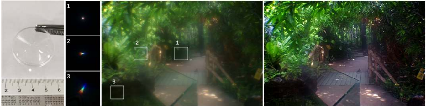
Fig. 1. Large Field-of-View Imaging With Thin-Plate Optics. We design a lens with compact form factor using one (or two) optimized refractive surfaces on a thin substrate (left). This optimization results in a dual-mixture point spread function (center-left insets), which is nearly invariant to the incident angle, exhibiting a high-intensity peak and a large, almost constant, tail. We show the sensor measurement (center) and image reconstruction (right) in natural lighting conditions, which demonstrate that the proposed deep image recovery effectively removes aberrations and haze resulting from the proposed thin-plate optics. Our prototype single element lens achieves a large field-of-view of 53^\circ with a clear aperture of f/1.8 and effective aperture of f/5.4 , see text.
