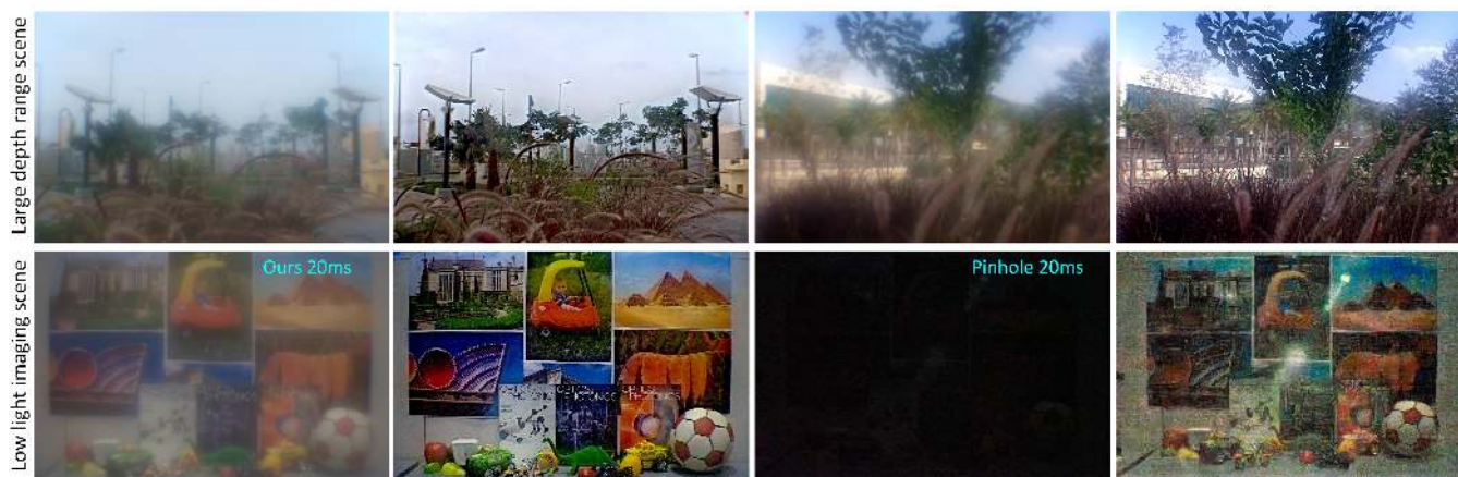
Fig. 12. Experimental results of large depth range imaging (top row) and low-light imaging (bottom row). The exposure time and ISO for the top two examples are set (3.125, 1) ms and ISO 50, while that for the bottom two examples are set (10 ms with ISO 500) and (20 ms with ISO 25,600).
