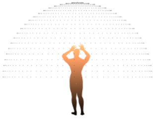
Fig. 3: Virtual cameras are placed on the hemisphere looking towards the center of the sphere to generate 108 virtual views.
