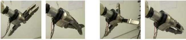
Fig. 2: Grasp preshapes. In this work, grasps are executed by setting the manipulator to either one of a parallel (first image) or cylindric (third image) preshape, then closing the fingers towards a goal configuration (second and fourth images) until resistance is encountered.
