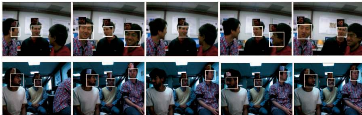
Fig. 13. Example tracking result in two test sequences. The first row is from sequence 1. The second row is from sequence 2. On top of each tracked face, a training example with the same face orientation is displayed. The tracker stops tracking when the left-right rotation of a face is larger than 90 degrees from a frontal face. A face is missed in the fifth example frame of the first sequence and the third example frame of the second sequence.
