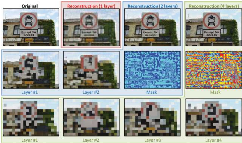
Figure 17: Reconstructions of an image under a field of masked RBMs with differing numbers of appearance layers. Each appearance layer is represented by a grid of nonoverlapping beta RBMs. In each case, the reconstruction uses 4 bits per pixel. The reconstruction quality is highest for K = 4 , indicating a good trade-off between representing appearance and shape of objects in the image. In the mask images, all superpixels belonging to the same grid have the same color.
