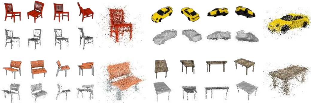
Figure 5: Qualitative results for per-view depth map prediction on ShapeNet. We show the depth maps predicted by Depth-LSM (visualized with shading from a shifted viewpoint) and the point cloud obtained by unprojecting them into world coordinates.
