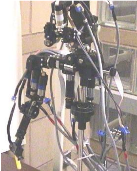
Fig. 1. The robot, Nico. Nico is an upper-torso robot with a 6-DOF arm (left) and a 7-DOF head. Its four CCD cameras are located on either side of the bottom of Nico’s “forehead” cylinder (top, left).
