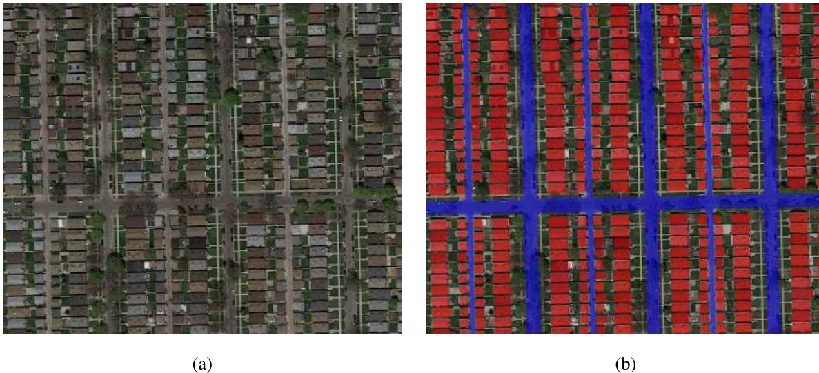
Fig. 5. FCN trained on Google Maps imagery and OSM labels of Chicago. (a) Original aerial image. (b) Overlaid with classification result.
