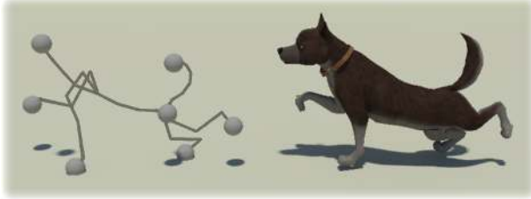
Figure 4: Result of Rig-space Full Body IK. From seven end effectors placed at four feet, head, hip, and tail, the optimal rig attributes are approximated by GPR and the solution is further refined by gradient descent. The animators can interactively pose the character using seven end effectors while the rig attributes are updated in real time.
