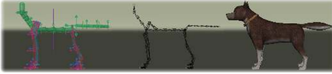
Figure 2: Typical setup of rigged character, showing animation rig, underlying skeletal structure, and mesh.
