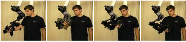
Fig. 8. Sarcos Master arm used to record a human trajectory in end-effector space. Here, the subject demonstrates a pouring movement which after learning the DMP enabled a robot to pour water into several cups (Fig. 12).
