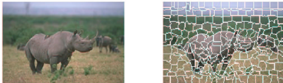
Fig. 2. An original image with 120x180 pixels becomes a 300 super-pixel image, where each contiguous region with a delineated boundary is a super-pixel
