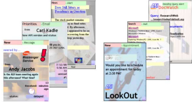
Figure 5. Sample visual alerts from Notification Platform, including news, financial alerts, email, instant messages, and output from services, such as a scheduling agent, background querying, and new document tracking. The service weighs the expected cost of interruption and the value of information in decisions about alerting and display modalities.
