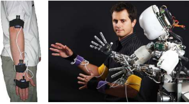
Fig. 7. Left : X-Sens motion sensors used to record the user’s gesture by collecting joint angle trajectories of the two arms (14 DOFs). Right : Demonstration of the skill with simultaneous reproduction on the robot.
