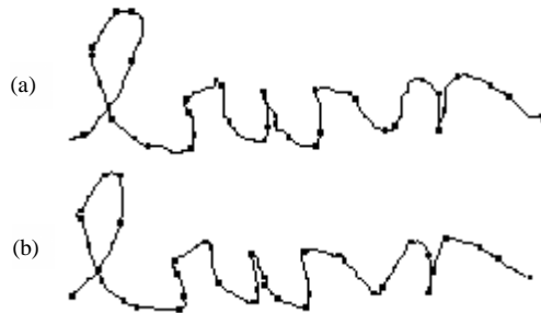
Figure 1. (a) Control points extracted from the original strait. (b) Reconstructed strait using control points and B-splines.
