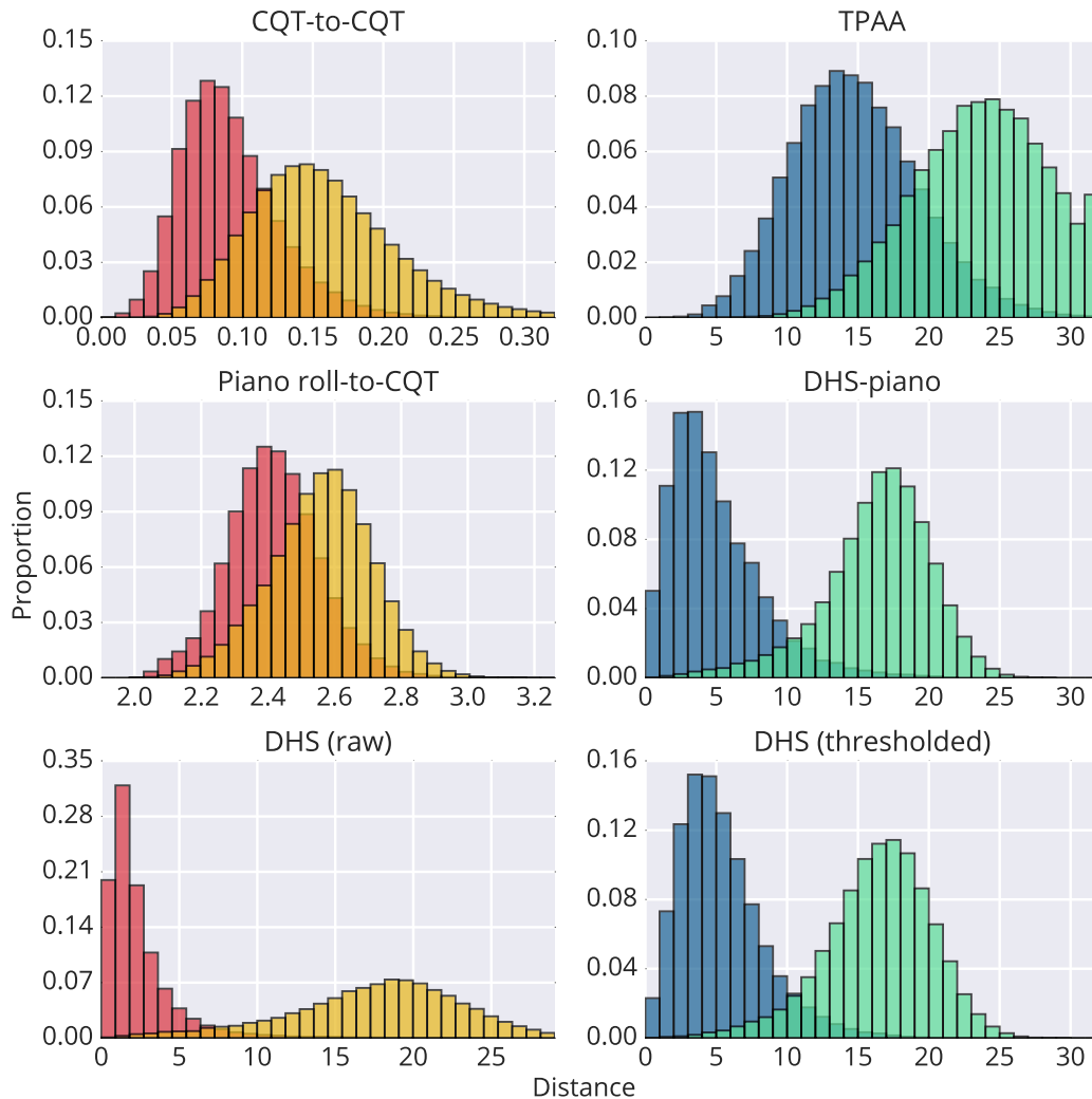
Figure 5.5: Distributions of distances for matching and non-matching sequence elements from our validation set for a variety of representations. Real-valued (squared Euclidean) distance distributions for matching and non-matching pairs are shown in red and orange respectively; Hamming distance distributions are shown in blue and green. From top left to bottom right are distance distributions for vectors produced by synthesized MIDI CQT-to-audio recording CQT, the TPA method, MIDI piano roll-to-audio CQT, the thresholded output of the DHS-piano model using this “multimodal” data, the DHS model prior to thresholding, and the DHS model after thresholding.
