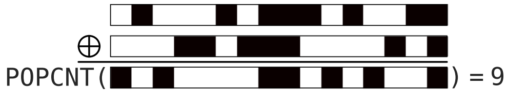
Figure 5.2: Computing the Hamming distance between two binary vectors via an exclusive-or followed by a POPCNT instruction. The exclusive-or of the top two vectors produces the bottom vector, which is 1 where the input vectors differ and 0 where they match. The result of the exclusive-or is passed to the POPCNT SSE4.2 instruction, which simply counts the number of non-zero bits in its input. These two steps therefore can produce the distance between two binary vectors in two machine instructions.
