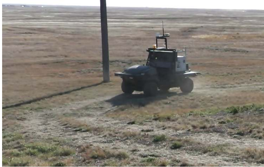
Figure 16: In experiment 3, we tested with a 600 kg, Ackermann-steered robot repeating a 100-m-long path. Like the previous experiments, the nominal model used by the LB-NMPC algorithm was a unicycle model, demonstrating the algorithm’s ability to be applied to robots with significantly different designs.
