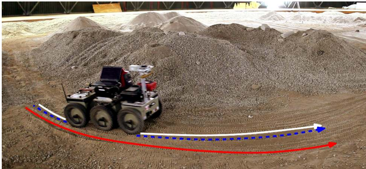
Figure 11: The second and third experiments focused on the algorithm’s ability to learn unmodelled robot dynamics. Here we show the skid steered ROC6 robot driving at 0.6 m/s with learning enabled. The white line shows the desired trajectory (tire tracks), the red line shows a trajectory with learning disabled, while the dashed blue line shows a trajectory with learning enabled and reduced path-tracking errors.
