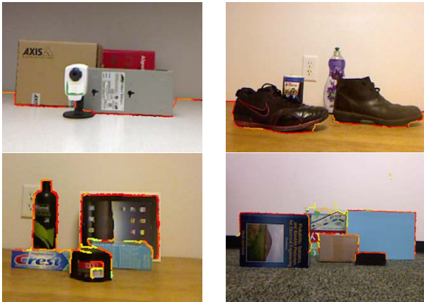
Fig. 4. Boundary detection result using the proposed algorithm. It reliably detects the connected (top two) and occlusion (bottom two) boundaries in different scenarios. The color indicates the confidence in classification. The more red it is, the larger the belief.
