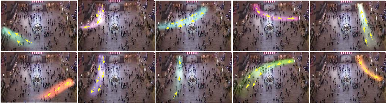
Fig. 11 Density distributions of ten exemplar semantic regions estimated from trajectories sampled from MDA.
