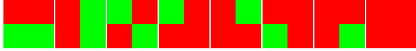
Figure 1. Eight 2 \times 2 checkerboard-like filters used in this work. Red (Green) is used to represent value +1 (-1).
