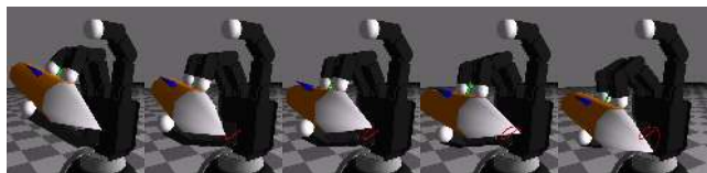
Fig. 12. Snapshots of generated writing motion on simulated Allegro hand
