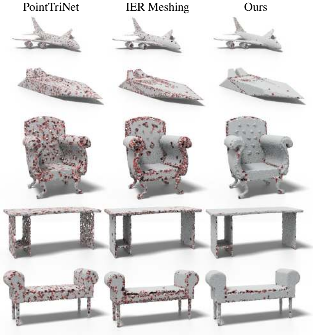
Figure 6. Qualitative comparison on ShapeNet [11]. We compare with the two data-driven methods PointTriNet and IER Meshing on five shapes taken from five different categories of the ShapeNet dataset. Our approach results in more manifold meshes, especially in detailed areas like the backrest of the chair.
