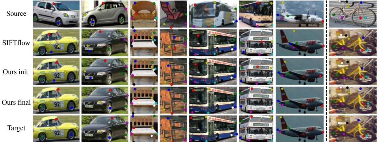
Figure 5. Comparison of keypoint transfer performance for different methods on example test image pairs. Overall, our consistency-supervised network (second-to-last row) is able to produce more accurate keypoint transfer results than the baselines. The last column shows a case when SIFT flow performs better than ours.
