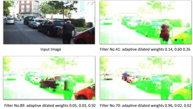
Figure 5. Visualization of active maps corresponding to different filters of block 3 of our D 4 LCN. Each filter learns three weights representing dilation rate of 1, 2, 3, respectively. Different filters have different functions in our model to handle the scale problem adaptively. For example, filter 89 has large receptive fields for large-scale cars, while filter 70 deals with the small-scale cars.
