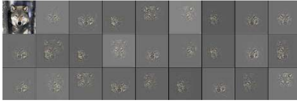
Fig. 4. The feature channels respond to target parts: images are reconstructed from conv5 of the CNN used in our tracker. Each image is generated by accumulating reconstructed pixels from the same channel. The input image is shown in the top-left.
