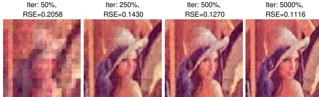
Figure 4: TR-SGD decomposition with TR-ranks of 12 on the 8th-order tensorization of an image. Iter: 50% indicates that only 50% elements are sampled for learning its TR representation. RSE indicates root relative square error \|\hat{\mathcal{Y}} - \mathcal{Y}\|_F / \|\mathcal{Y}\|_F .
