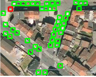
Figure 2: Aerial car detector. Left: example detections (correct in green, incorrect in red). Middle: precision-recall curves in the style of the PASCAL VOC challenge [5] for the linear and slot kernel structured SVM detectors and their equivariant versions. Right: FPPI vs recall curves for the different methods, including the method from [8] denoted as “context”.
