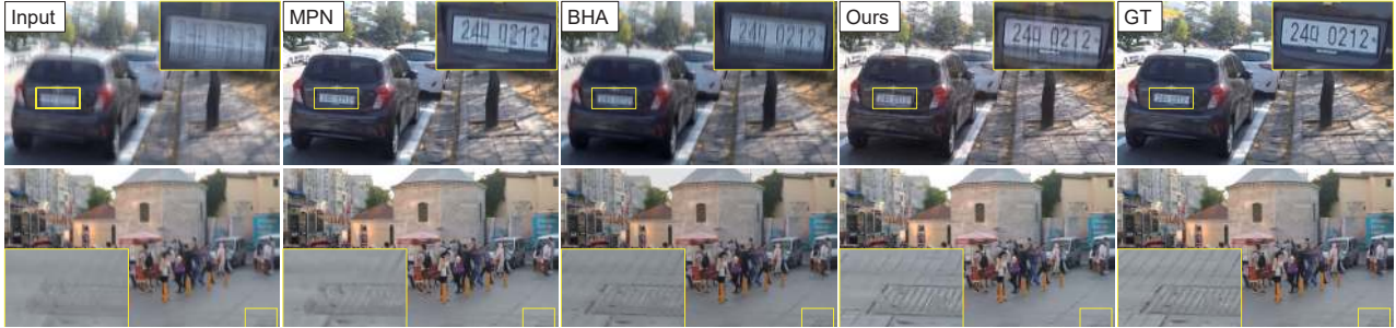
Figure 4. Visual comparisons on the GoPro dataset. From left to right, we show two examples with the blurred image, results of MPN [50], BHA [31] and our approach, as well as groundtruth sharp image, respectively. Zoom in for better view.
