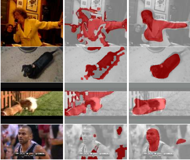
Figure 6. From left to right: a video frame, the output of uNLC that we use to train our ConvNet, and the output of our ConvNet. uNLC is able to highlight the moving object even in potentially cluttered scenes, but is often noisy, and sometimes fails (last two rows). Nevertheless, our ConvNet can still learn from this noisy data and produce significantly better and smoother segmentations.
